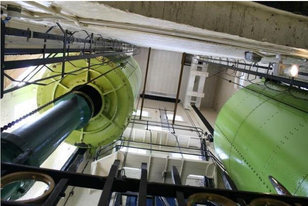
These accumulators stored pressurised water and were filled with water by the water pump on the steam pumping engine.
