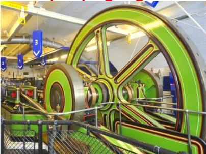
These machines used the steam from the boilers to power a water pump which you can see when you reach the other end of the engine.
